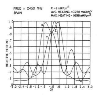
Figure 1. Absorbed energy pattern along the rectangular coordinate axes of a 3.0 cm spherical head exposed to 2450 MHz radiation (13). The incident power is 1 mw/cm<sup>2</sup>.
