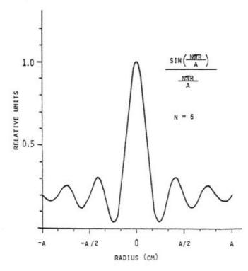
Figure 3. Approximated spherically symmetric absorbed energy pattern in a spherical head model.
